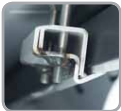
Bolt-on brackets quickly secure Slide-In bodys
