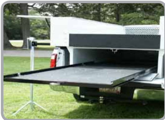
FlexSmart Deck Slide provides easy access to cargo under the bed floor
