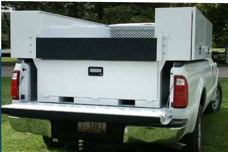
Bolt-on brackets quickly secure Slide-In bodys
